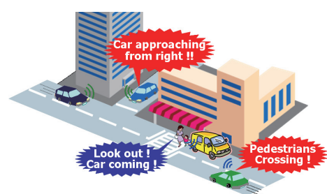
Wireless communication between vehicles and pedestrians to warn of collision dangers.
